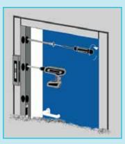
To fit the bottom aluminium sill (where applicable), drill and fit to the floor.
