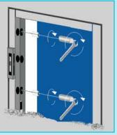
A Hex Tool is supplied to tighten adjusters.
